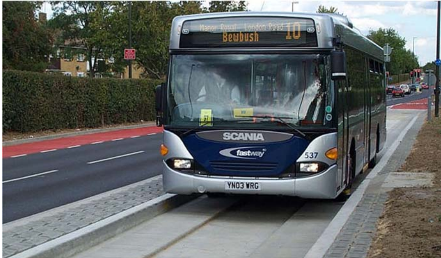
Figure 6: Fastway guided busway
